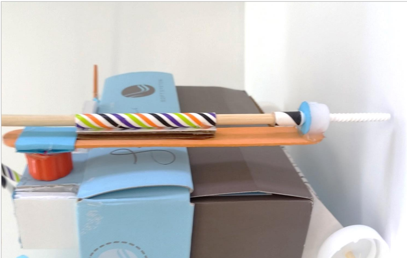
Drill System: glue stick screw and nut, skewer axle, straw bearing, attached to popsicle stick lever arm, connected to wheel and axle mount from plastic cap
