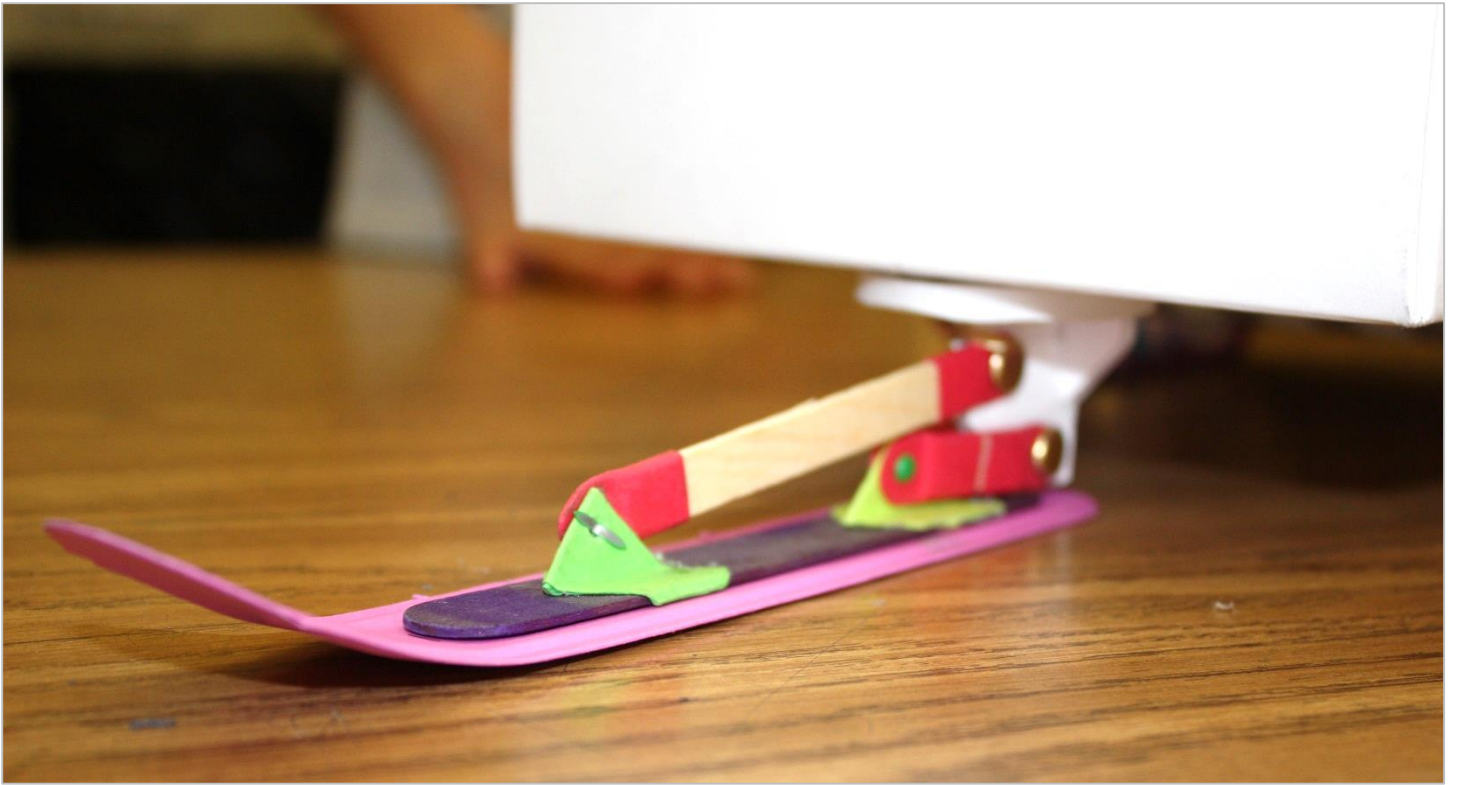
Ski Assembly: swivel mount holds lever system attached to ski stabilized with popsicle stick
