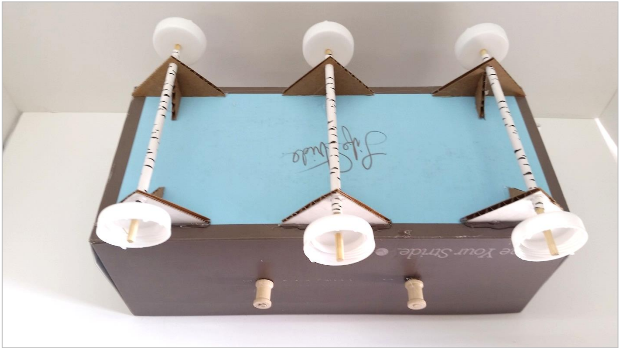
Wheel and Axle System: straw bearings, skewer axles, foam core braces and struts, lid wheels
